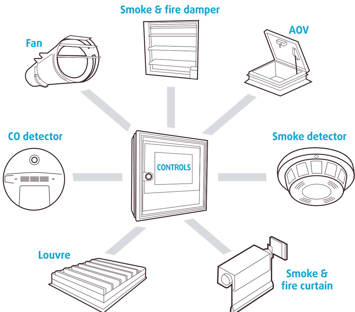
Failure of a single element can throw the effectiveness of the whole life safety system into doubt. Airvent engineers don't just know how to maintain or repair single elements; they understand how the elements work together and test systems accordingly.
